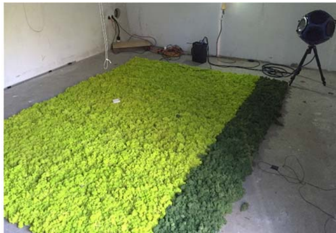
Figure 1 - 5.93 m 2 Mossart, 18 Large panel, 5 small panel assembly
